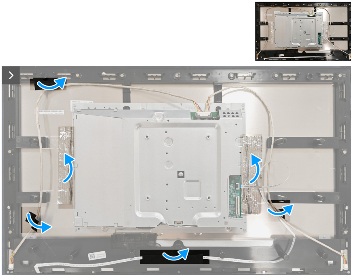
Figure 20. Removing the metal shield
