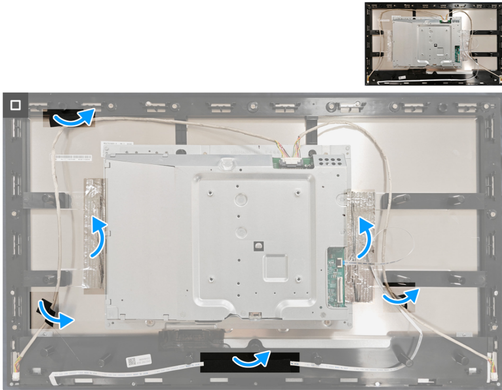
Figure 29. Installing the metal shield
