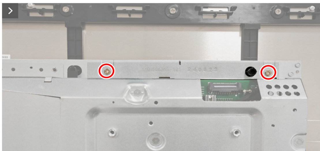
Figure 26. Installing the metal shield
